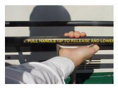
**Step 3:** To release the rack, squeeze the center handle and slowly lower it. If the rack is already lowered and a bike is in position, use the other available bike wheel well. If the bike rack is full, please wait for the next available bus.
